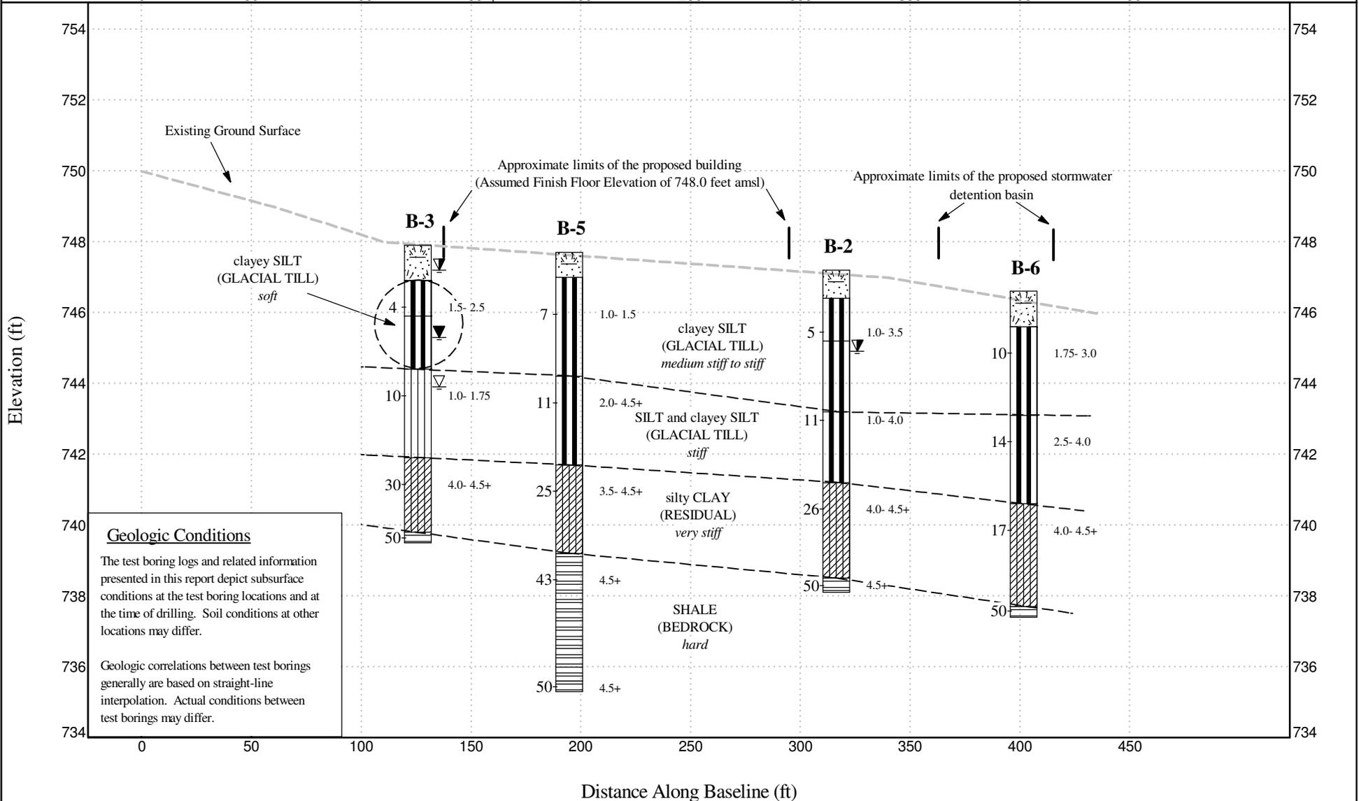
STRATIGRAPHY & GW - A SIZE 161-305 DRAFT BORING LOGS.GPJ GOOD TEMPLATE.GDT 3/20/18
