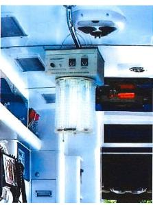
The EDU-435 has a built in full metal handle so it can be inverted inside the ambulance from ceiling rails or hooks.
